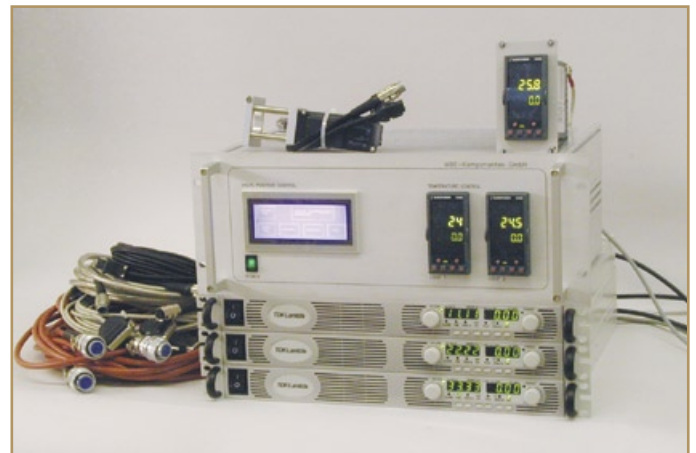
Additional equipment for the VCCS (motorized valve control unit MVCU with temperature controllers, power supplies and cables)
