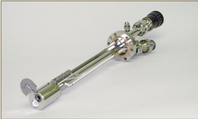
Dual Dopant Source DCS 40-2x1-14-S Two 0.6cc PBN crucibles on one flange DN40CF (O.D. 2.75"), with integrated water cooling surrounding the heaters
