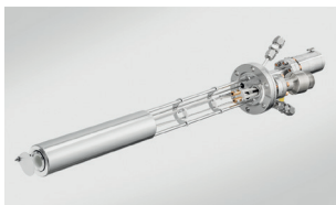
Effusion cell 2 to 10 cm 3 , high temperature cell
